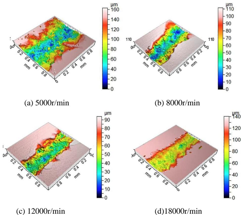
Fig. 4 The 3D topography of fused silica glass surface with different grinding wheel speeds
