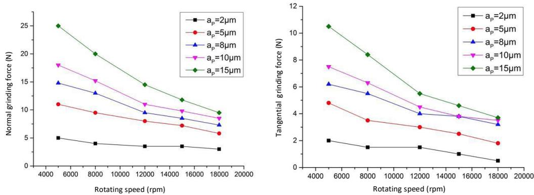
Fig. 3 The Normal and tangential force of the grinding experiment with different rotating speed
