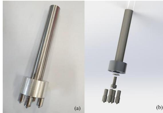
Fig. 1 The diamond tool for single grain grinding test: a) the picture of the diamond tool, b) the component diagram of the diamond tool.
