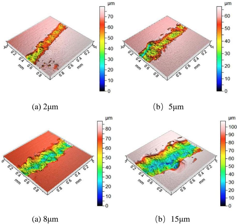
Fig.5 The 3D topography of fused silica glass surface with different grinding depth
