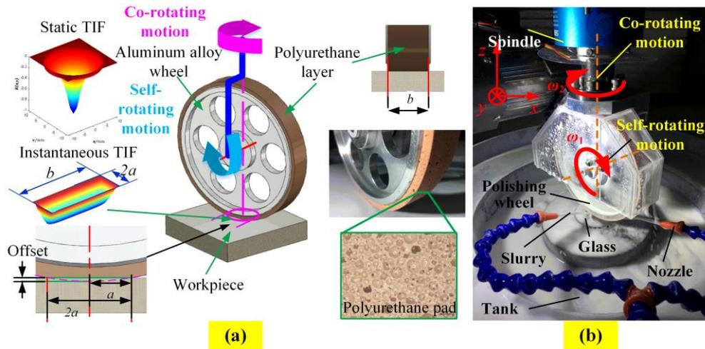
**Fig. 1.** Illustration of the DAWP system (a) schematic diagram of the semi-rigid polishing wheel; (b) photograph of the DAWP tool during polishing process.
