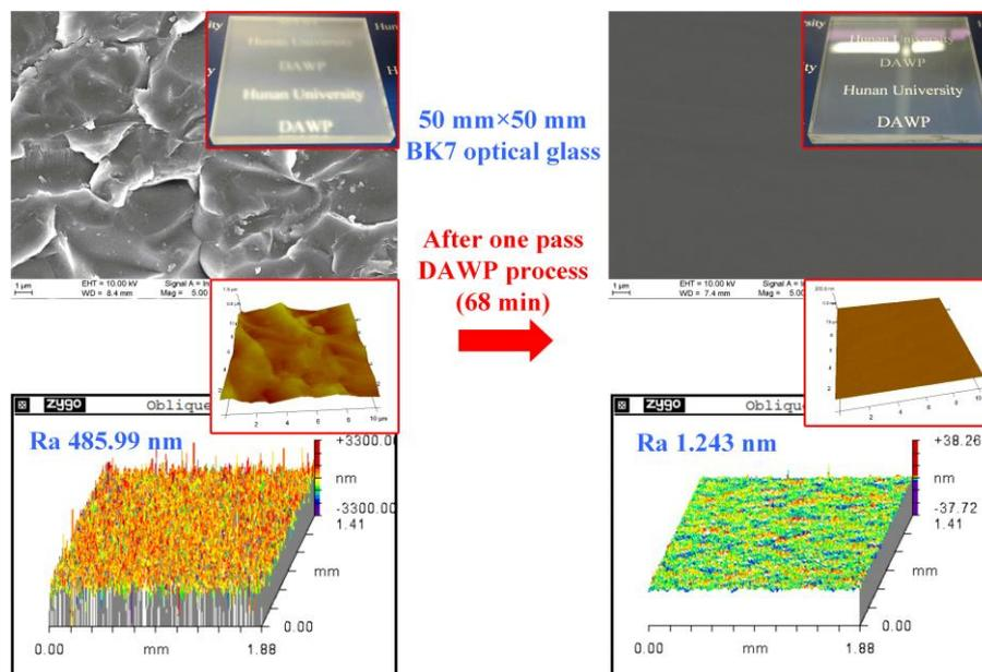
**Fig. 4.** Surface topography, roughness and appearance of BK7 flats before and after one pass polishing.
