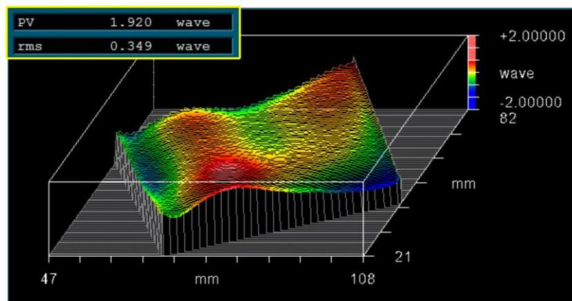
**Fig. 5.** Measured surface form error of 50 mm×50 mm BK7 flat after one pass polishing.
