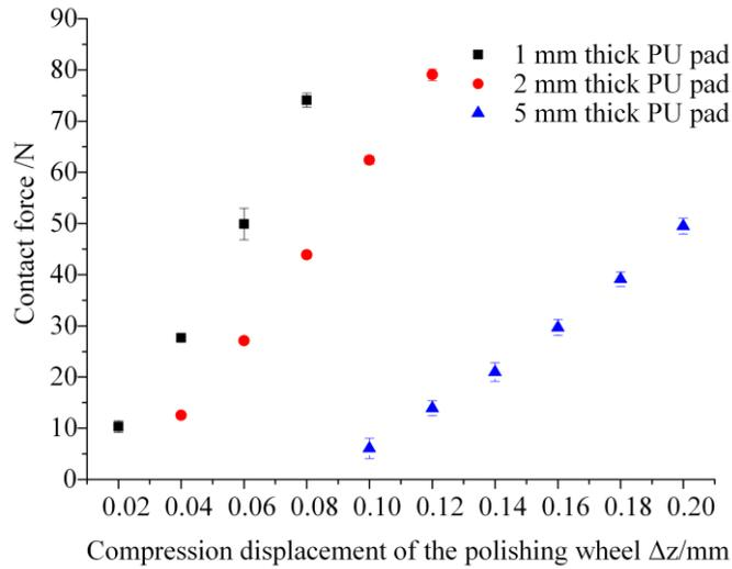
**Fig. 3.** Measurement results of the polishing contact force.
