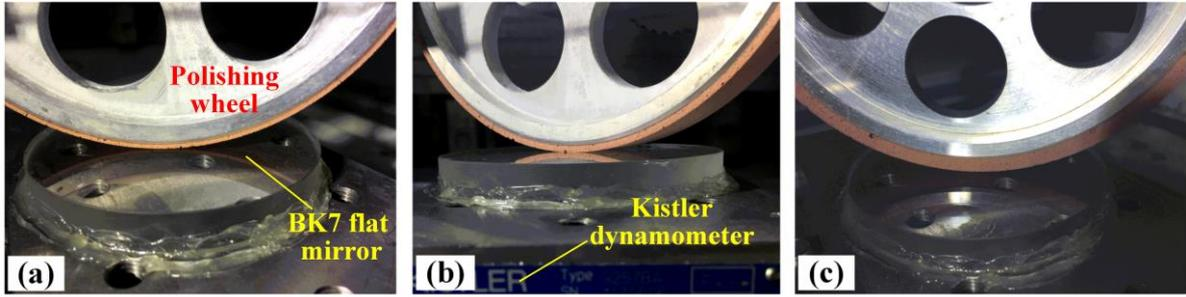
**Fig. 2.** Contact force measurements for the polishing wheel with different PU thickness (a) 1 mm (b) 2 mm (c) 5 mm.
