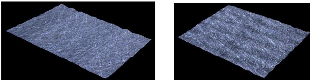
(a) Spindle rotation speed 1200 [rpm] (b) Spindle rotation speed 6000 [rpm]
