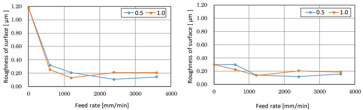
(a) Result of roughness along to the x direction (b) Result of roughness along to the y direction
