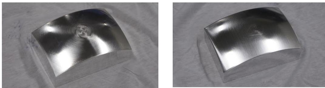
(a) Surface used by contour tool path      (b) Surface used by scanline tool path
