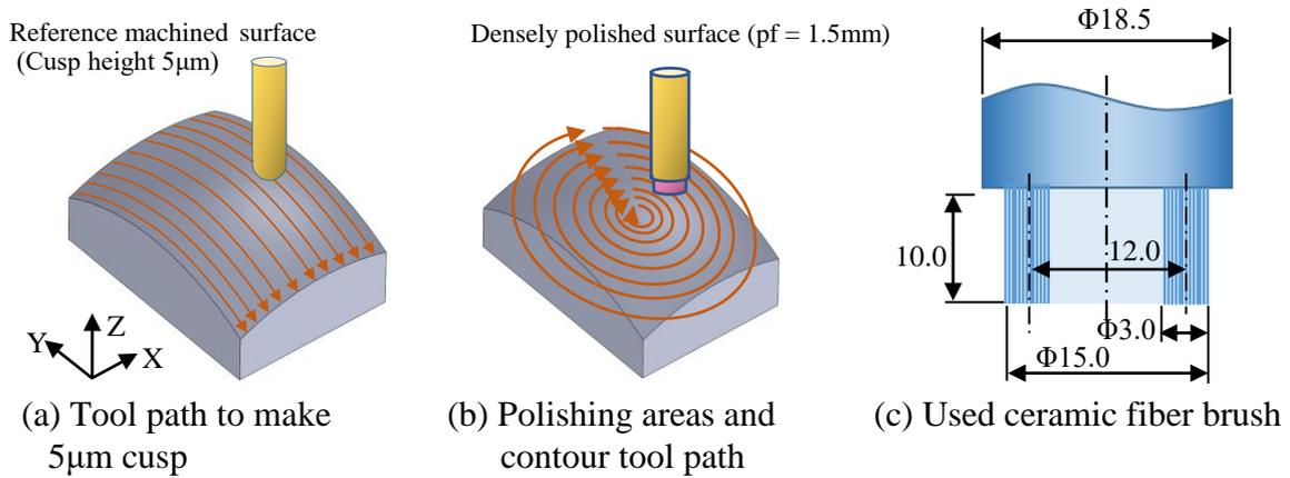
Figure 3. Process of polishing using contour tool path to a spherical surface and used ceramic fiber brush
