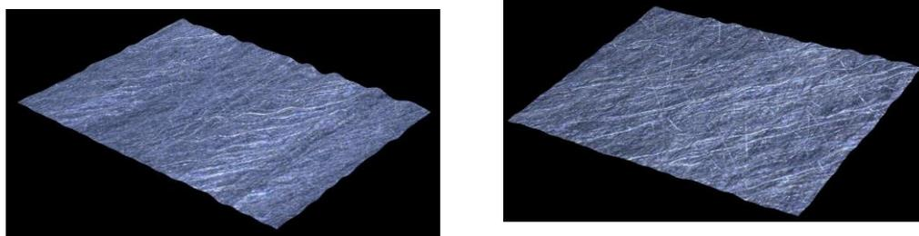
(a) Feed rate 600 [mm/min] (b) Feed rate 3600 [mm/min]
