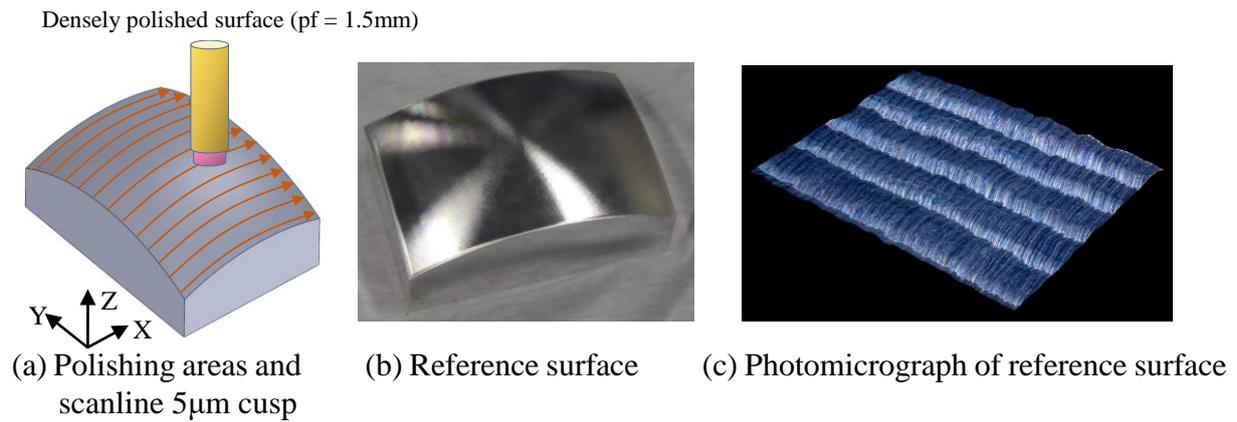
Figure 5. Process of polishing using scanline tool path and reference surface
