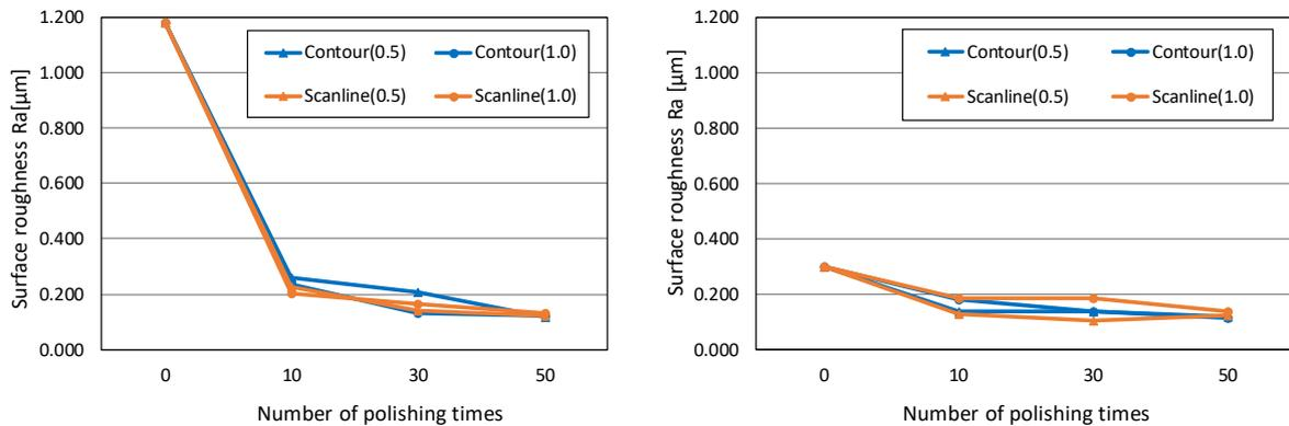
(a) Result of roughness along to the x direction      (b) Result of roughness along to the y direction
