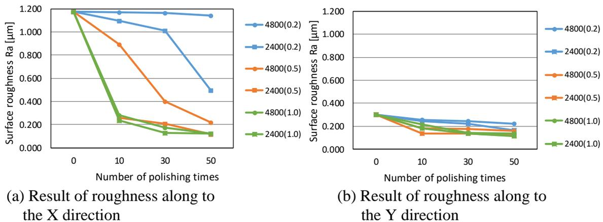
Figure 4. Measured surface roughness of spherical surface using contour tool path
