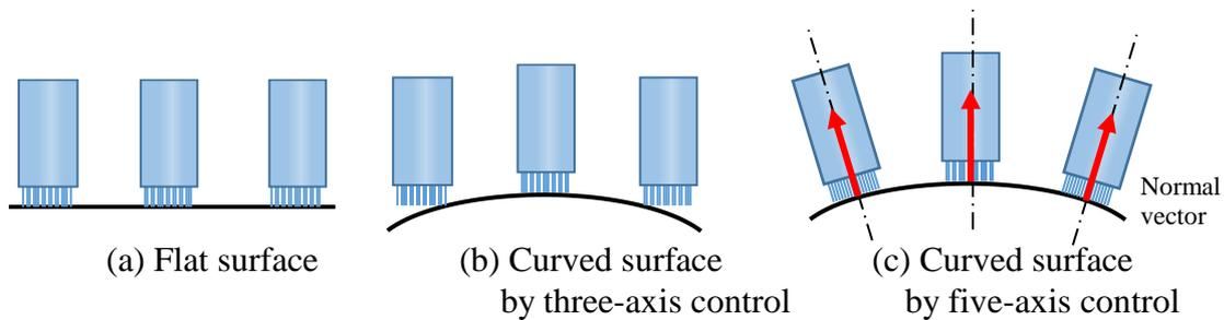
(a) Flat surface (b) Curved surface by three-axis control (c) Curved surface by five-axis control
