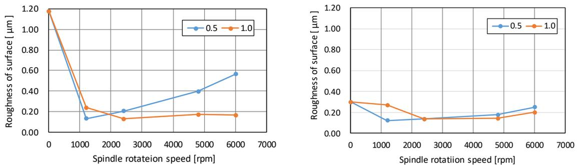
(a) Result of roughness along to the x direction (b) Result of roughness along to the y direction
