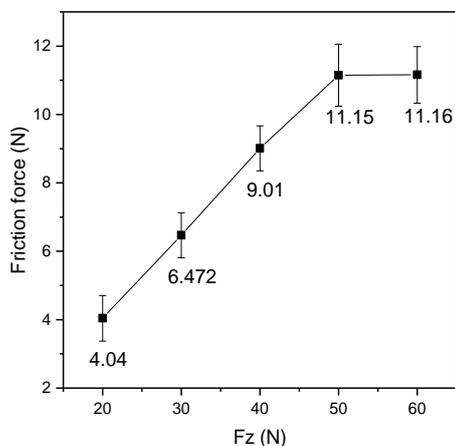
**Figure 2** Coefficient of friction under different loads
