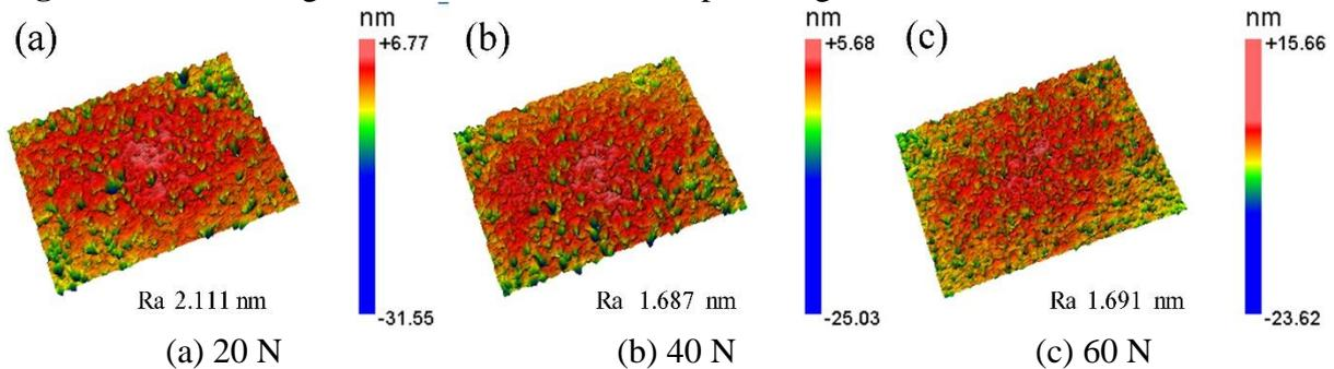
In order to verify the conjecture in the friction experiment that different loads lead to different diamond surface quality, three loads with the value of 20 N, 40 N and 60 N were selected as the polishing load for CMP. Figure 5 and Figure 6 show the morphology and surface roughness of diamond surface after polishing respectively.
