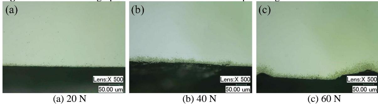
**Figure 6** Surface roughness of the diamond after polishing under different loads
