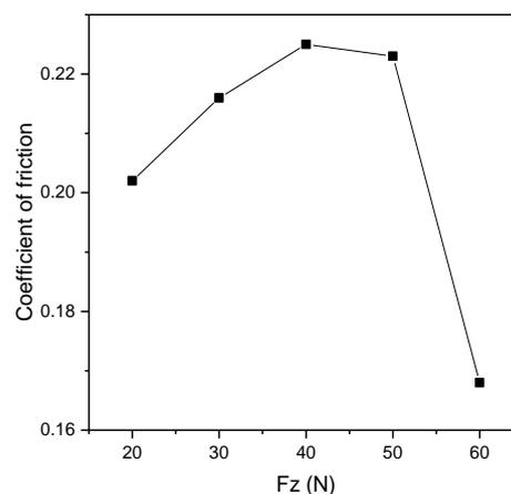
However, when the value of load is higher than 40 N, the friction force has no significant change with the load increase. The friction force is no longer proportional to the load. It indicates that the coefficient of friction  $\mu$  at the interface has changed according to Eq. 1. Coefficient of friction of interface under different loads is showed in Figure 2. It shows the coefficient of friction begins to decrease under the load of more than 40 N.
