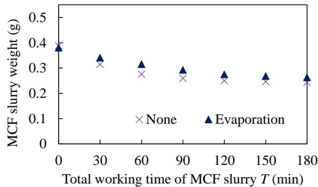
Fig. 4 Changes of the MCF slurry weight in each condition
