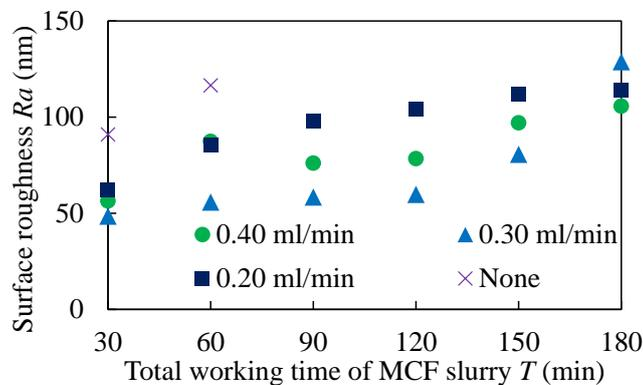
Fig. 3 Changes of the surface roughness in each condition
