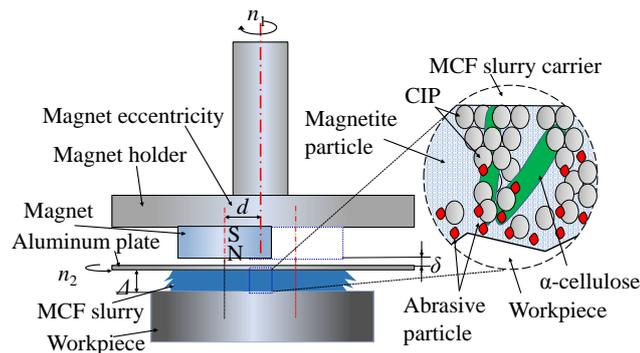
Fig. 1 Illustration of the ultrasonic vibration assisted MCF polishing process
