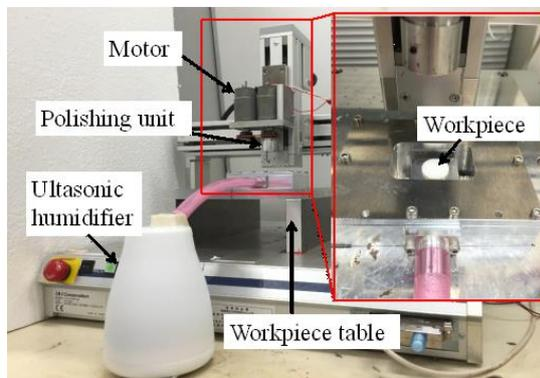
Fig. 2 Photograph of the experimental rig
