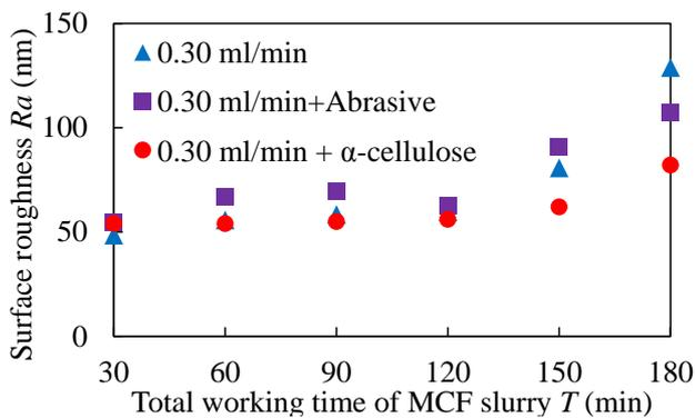
Fig. 5 Changes of the surface roughness in each condition
