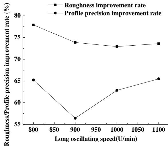
Fig. 3 Effect of long oscillating speed on roughness/profile precision improvement rates
