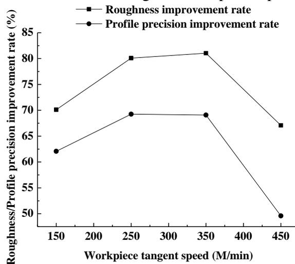
Fig. 1 Effect of workpiece tangent speed on roughness/profile precision improvement rate
