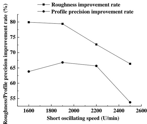
Fig. 4 Effect of short oscillating speed on roughness/profile precision improvement rates
