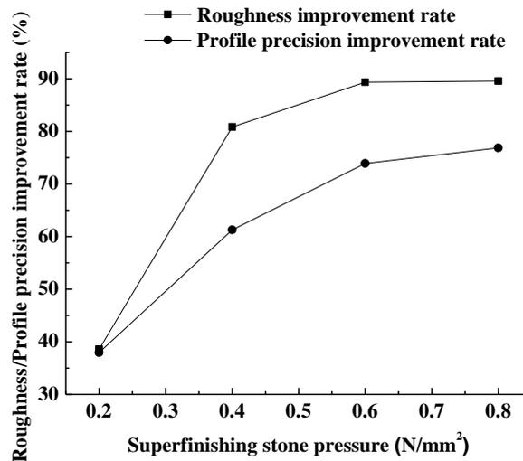
Fig. 2 Effect of superfinishing stone pressure on roughness/profile precision improvement rates
