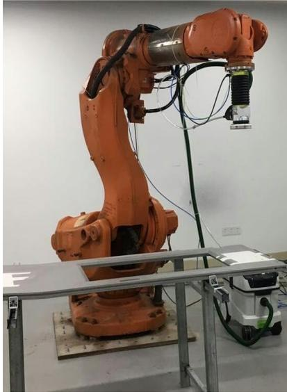
Fig.8 Automatic polishing system
