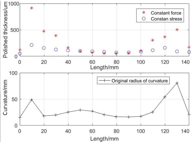
Fig.9 Result between constant force and constant contact stress
