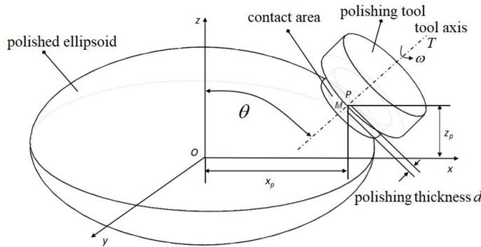
Fig.6 Geometric sketch of polishing
