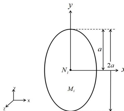
Fig.2 Elliptical contact area
