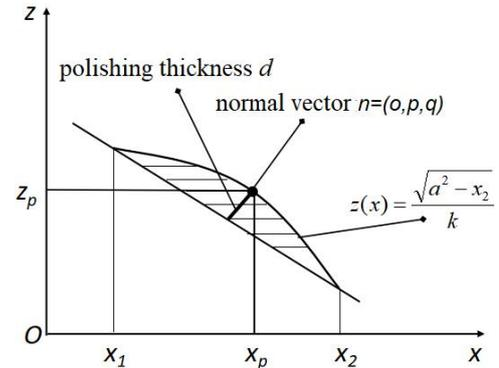
Fig.7 Analysis of cross section
