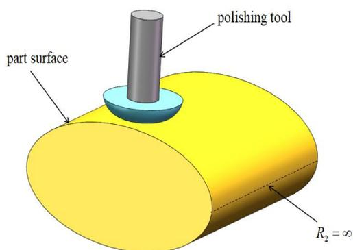
Fig.1 Polishing tool and part
