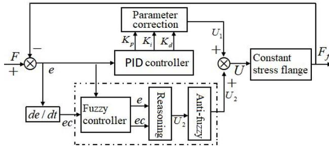
Fig. 4 Close loop control block diagram
