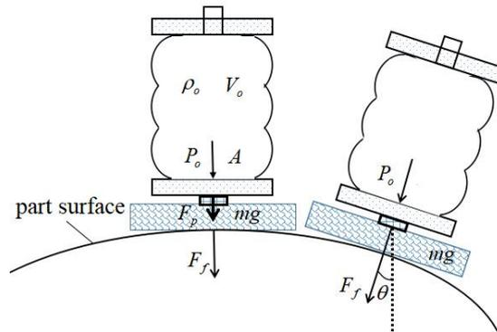
Fig. 3 Force analysis of flange
