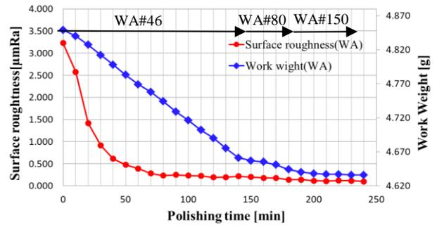
Fig.5 Polishing experiment result (WA)
