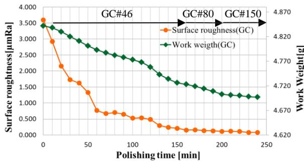
Fig.4 Polishing experiment result (GC)
