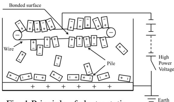
Fig. 1 Principle of electrostatic flocking method.
