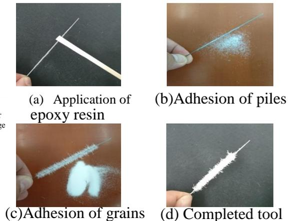
Fig. 2 Tool manufacturing
