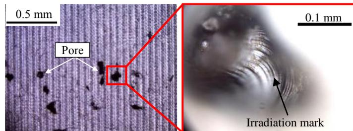
Fig. 3 Microscopic images of ball end-milled surface.
