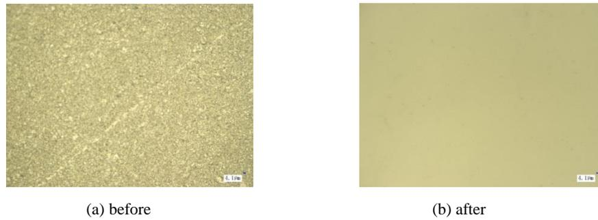
Fig.8 ultra-depth of field microscope (HIROX) in the workpiece surface before and after FRP
