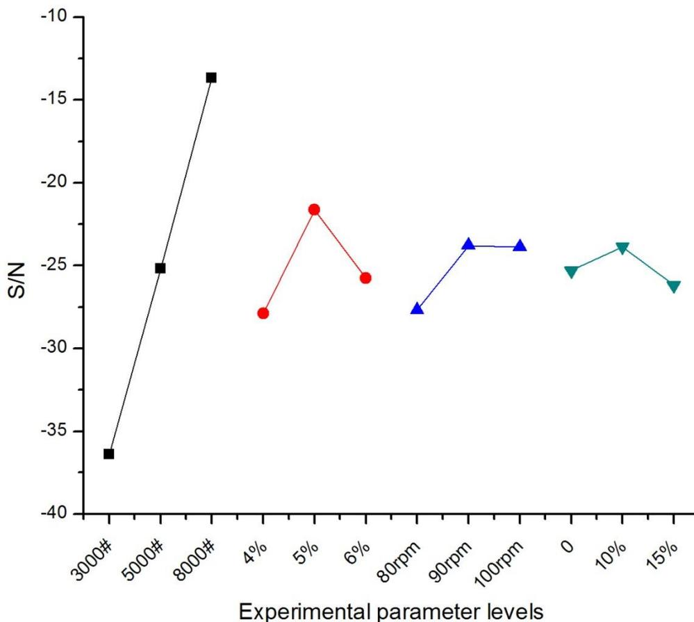
Fig.4 Plots of S/N ratio of each parameter level on  $Ra$
