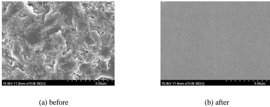
Fig.9 SEM micro-topographies of the workpiece surface before and after FRP
