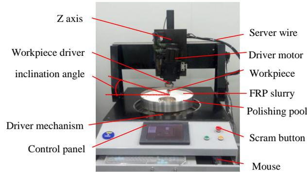
Fig.3-Experimental device for FRP
