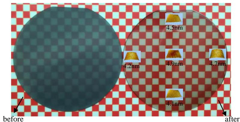
Fig.7 The  $LiTaO_3$  substrate before and after FRP
