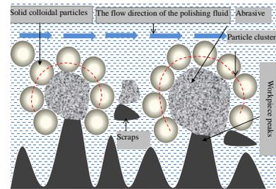
Fig.1-Schematic illustration of FRP Principle      Fig.2-Micro schematic illustration of FRP material removal
