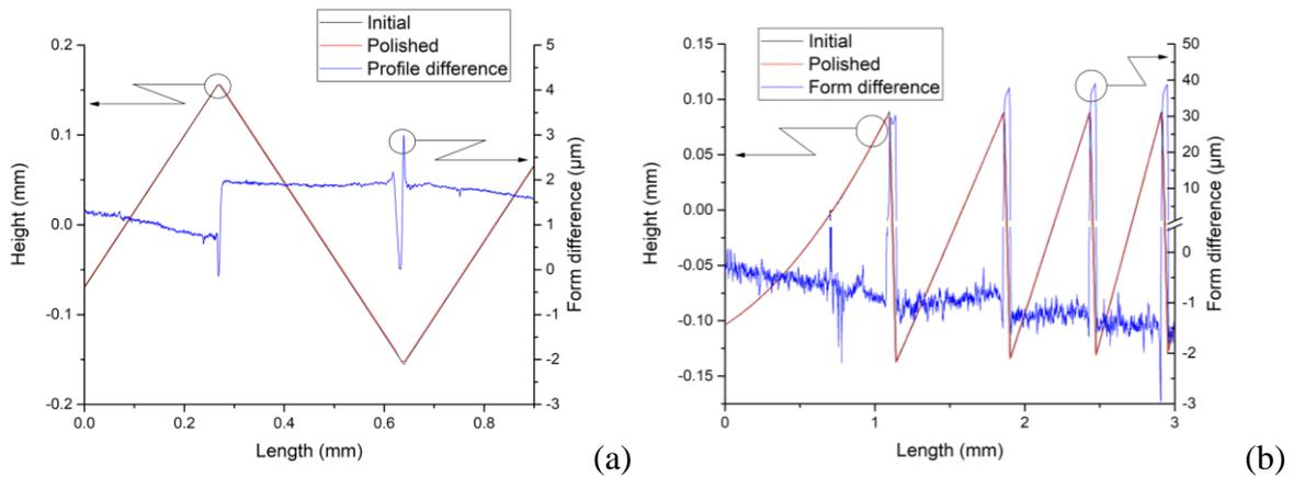
**Figure 5.** Form change of (a) V-groove and (b) Fresnel-type structures before and after polishing.
