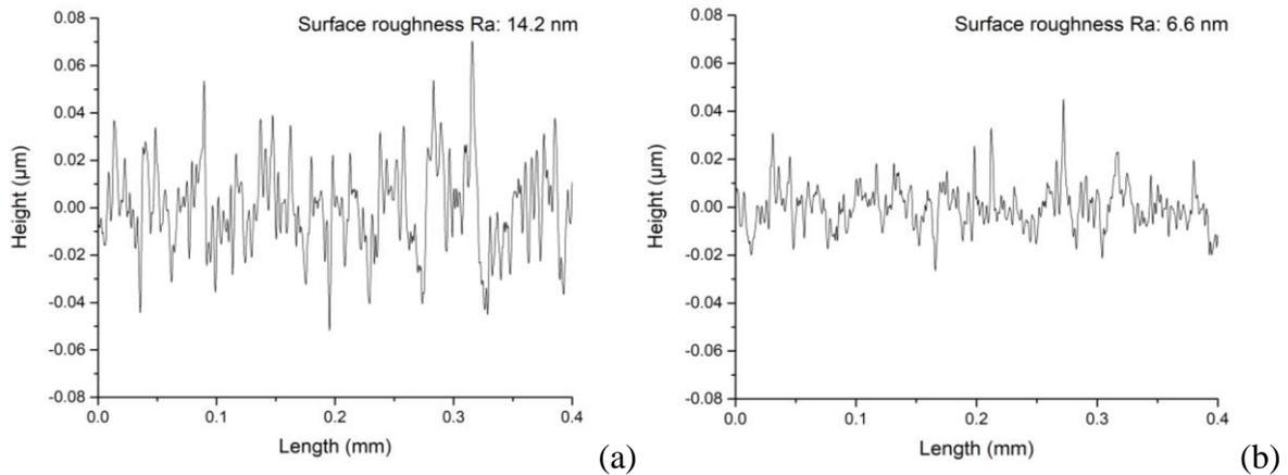
**Figure 3.** Surface roughness of V-groove structures (a) before and (b) after polishing.
