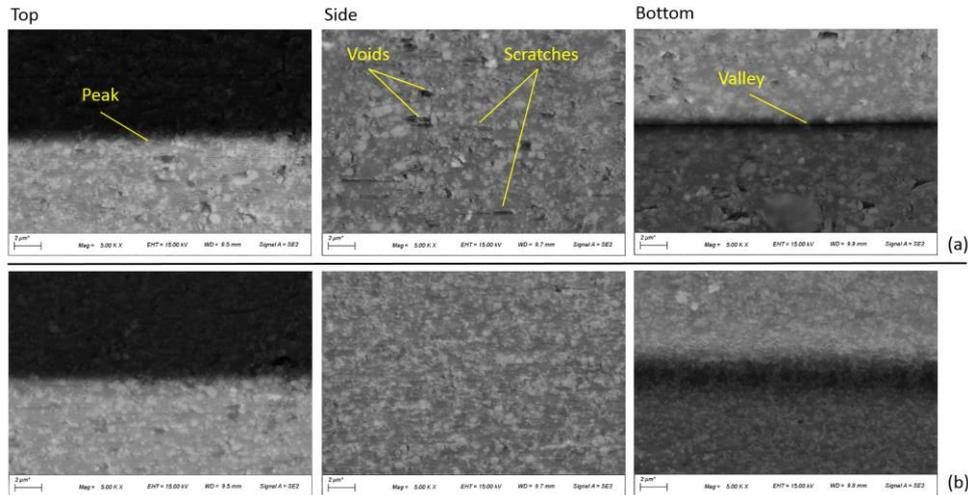
**Figure 6.** Secondary electron images of surface morphologies on top, side and bottom of V-groove structures (a) before and (b) after polishing.
