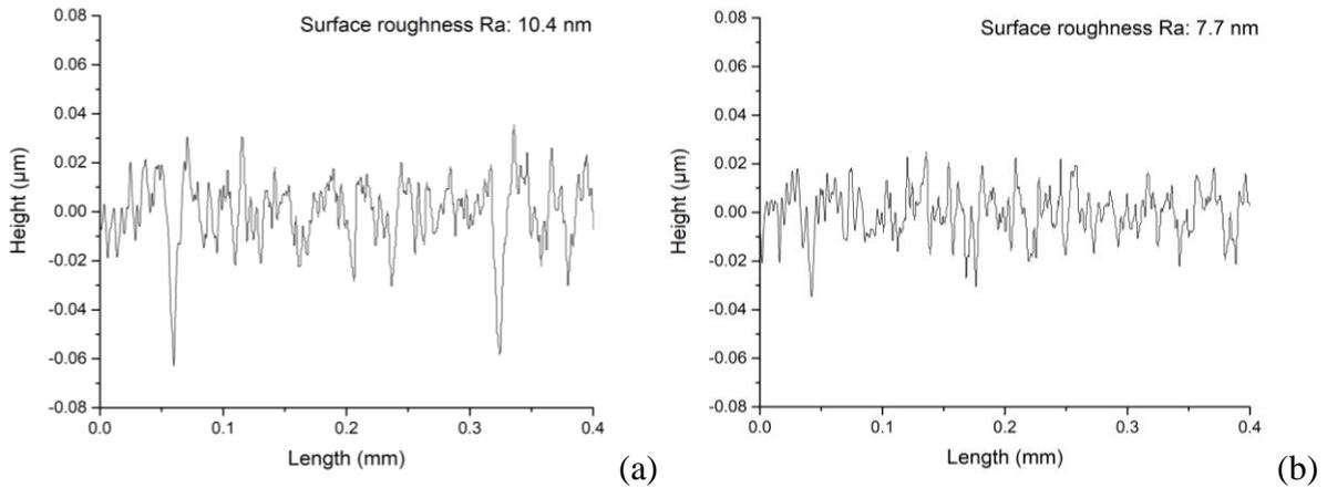
**Figure 4.** Surface roughness of Fresnel-type structures (a) before and (b) after polishing.
