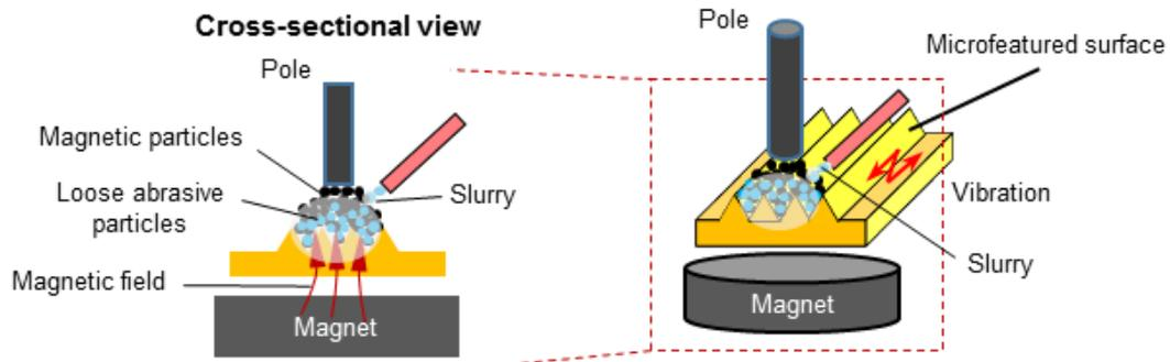
**Figure 1.** Schematic illustration of the VAMAP method.
