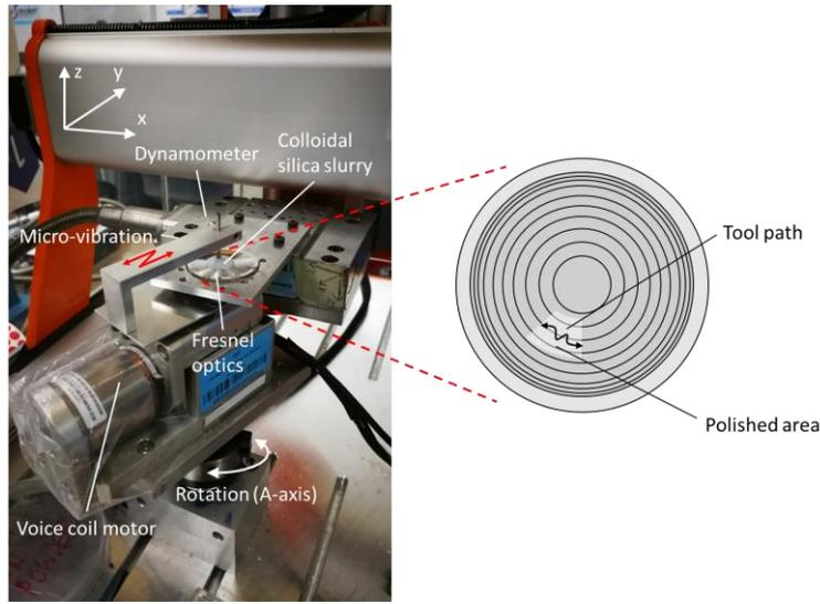
**Figure 2.** Experimental setups for (a) pole-magnet positioning, (b) V-groove and (c) Fresnel optics polishing.
